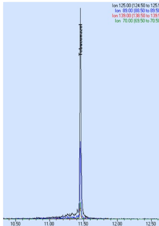
Tebuconazol, SRM mode I Group containing 4 SRM transitions: m/z 250>125, 125>89, 250>139, 250>70
