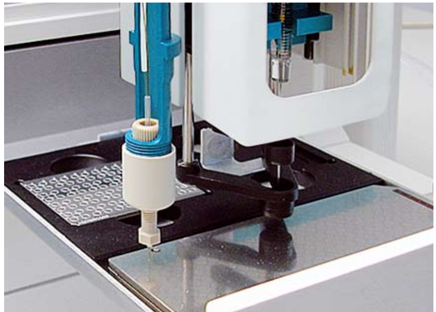
Fraction collection onto Maldi target
