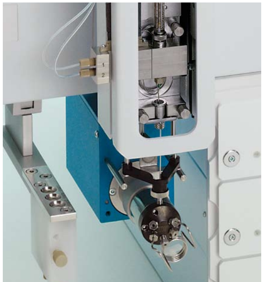
PAL HTS-xt equipped with DLW Option and a 6 port Injection valve (1000bar)
